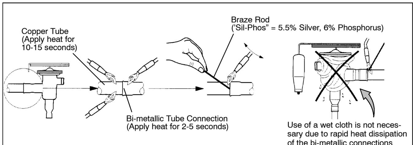
**Figure 6-21 Hermetic Thermostatic Expansion Valve Brazing Procedure**
