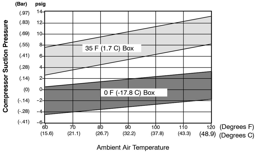
Compressor Suction Pressure Versus Ambient Air Temperature at Stable Box Temperature
