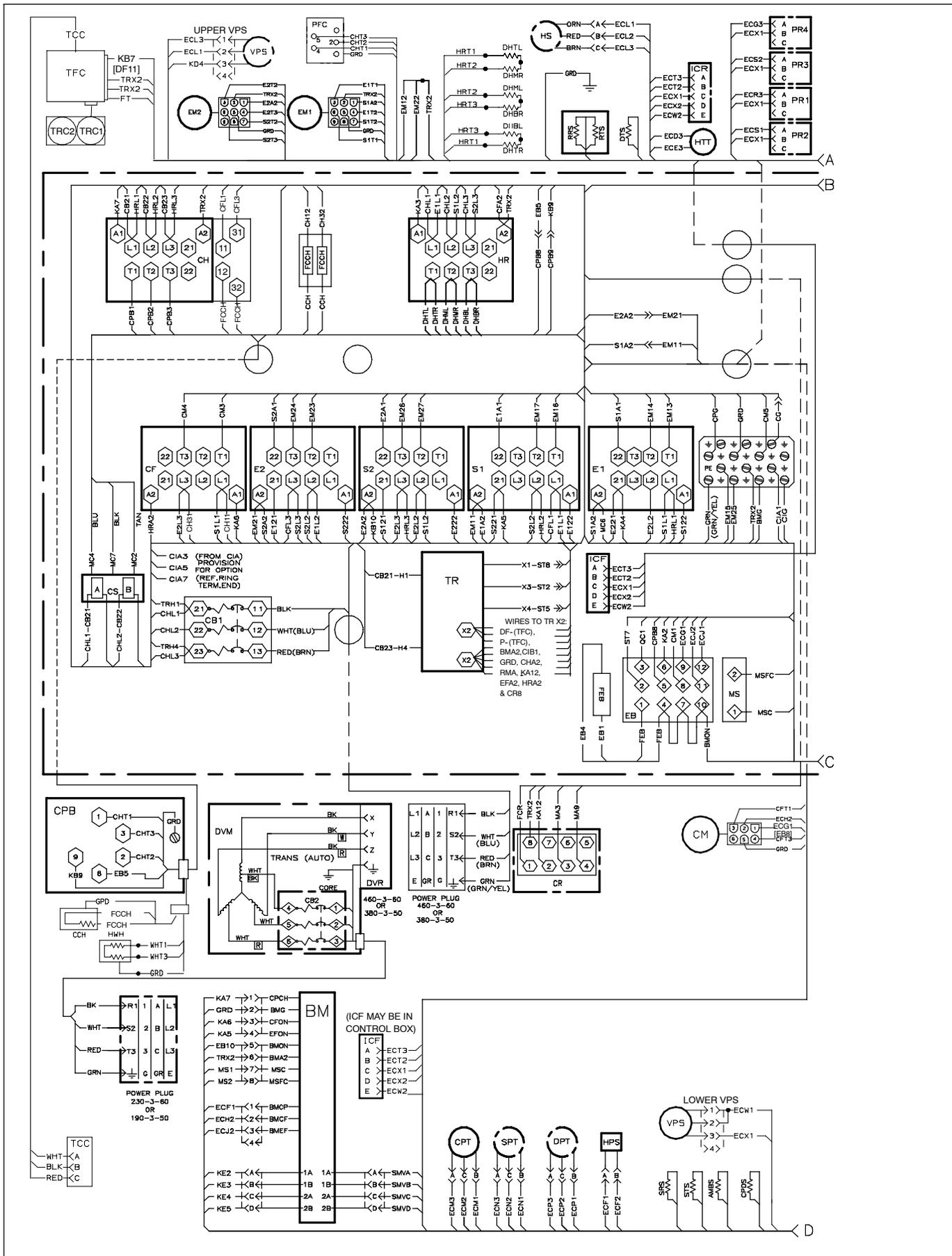
Figure 7-8 UNIT WIRING DIAGRAM - Units with Single Evaporator Fan Capability (Sheet 1 of 2)
