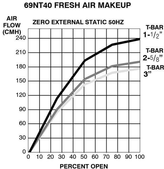
Figure 4-2 Make Up Air Flow Chart
