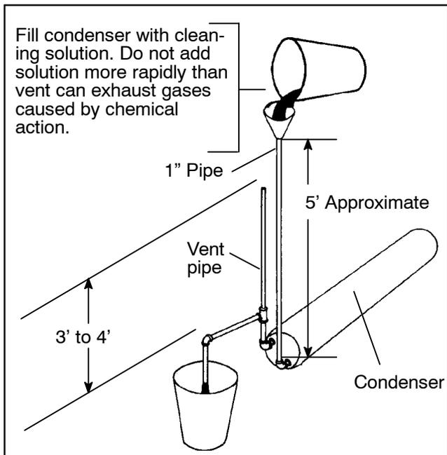
**Figure 6-18 Water Cooled Condenser Cleaning - Gravity Circulation**
