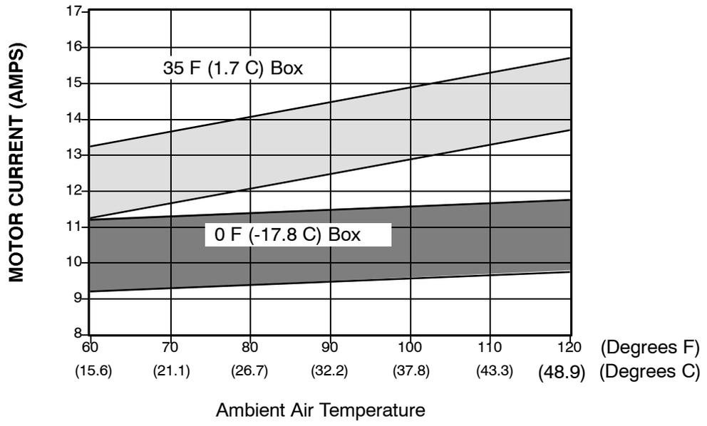
Compressor-Motor Current Versus Ambient Air Temperature At Stable Box Temperature
