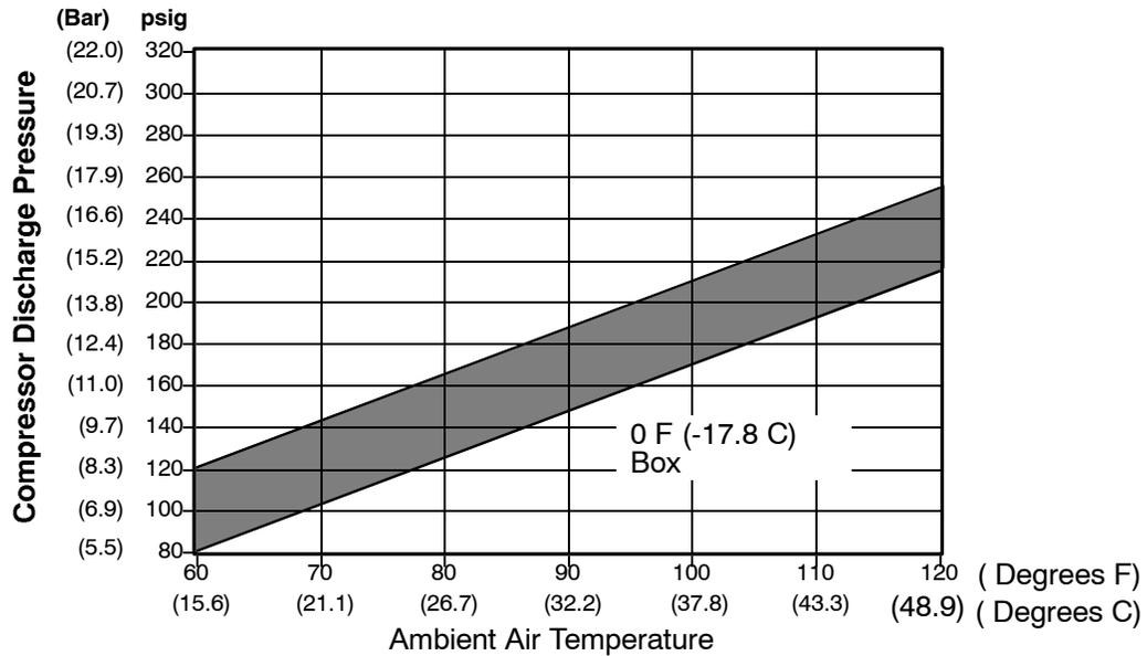
Compressor Discharge Pressure Versus Ambient Air Temperature at Stable Box Temperature
